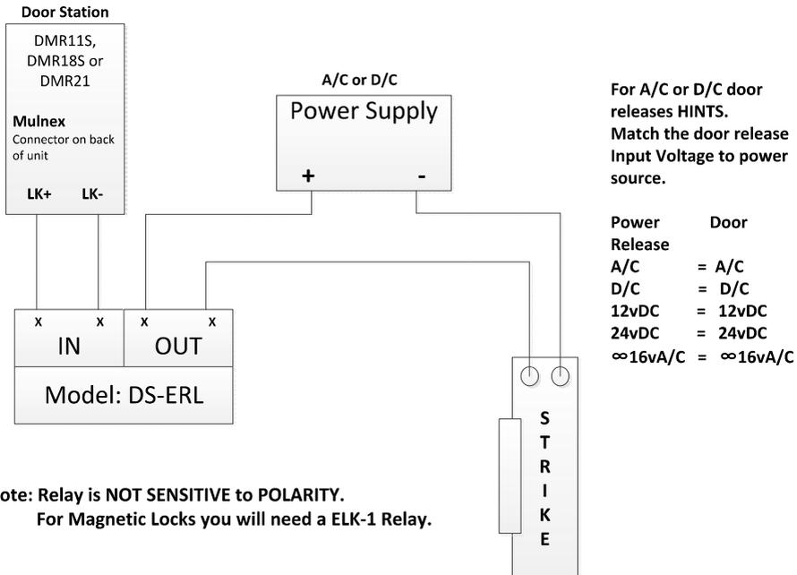
**Note:** Relay is NOT SENSITIVE to POLARITY.
