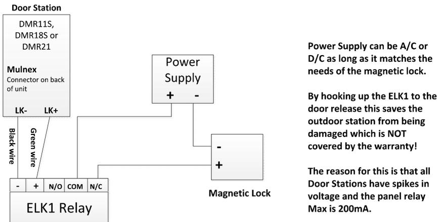
**Note:** The mulnex Connector is located on the back of the outdoor station, and the black wire used for the connection is the second wire from the top next to the green wire.
