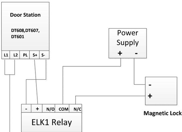
Power Supply can be A/C or D/C as long as it matches the needs of the magnetic lock.
